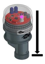
Once a large enough impact has occurred, the menu LED will then light up purple momentarily. Shortly after, the LED will blink twice (in blue or red) to indicate subsequent impacts are required to fully turn on the unit. By impacting the trigger twice more, the trigger turns on. For every impact the menu LED will light up purple. If the shock due to impact is
